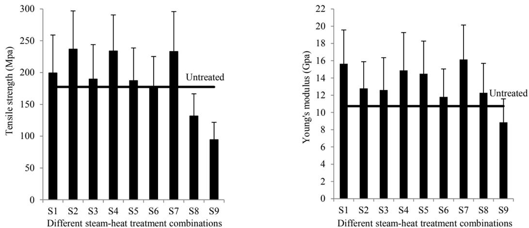
**Fig. 4** Mechanical strength of steam-heat treated flax fibres comparison among difference treatment combinations
