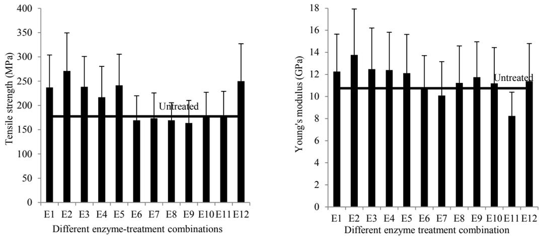
**Fig. 3** Mechanical properties of enzyme-treated flax fibres - comparison among different treatment combinations
