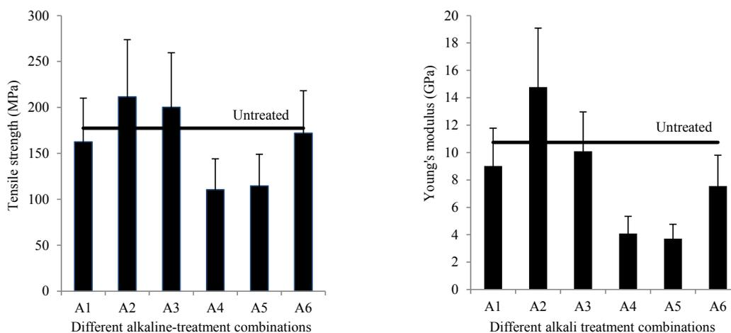
Fig. 2 Mechanical strength of alkaline-treated flax fibres - comparison among different treatment combinations
