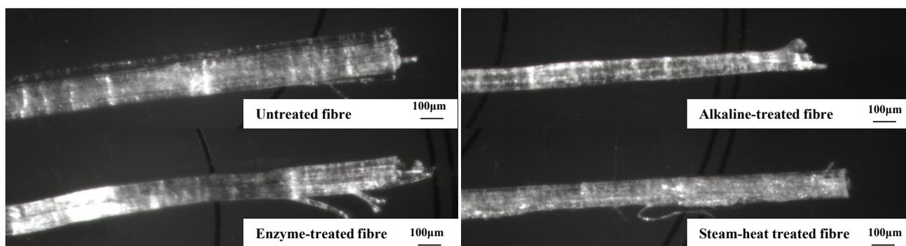
**Fig. 1** Diameter measurement of untreated and treated flax fibres observed under optical microscopy
