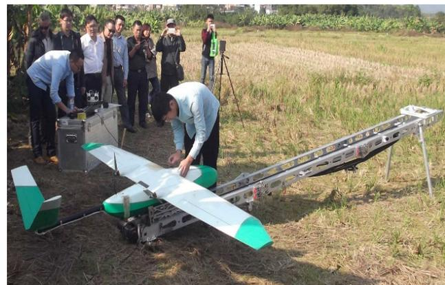
**Fig. 6** Take-off preparation of the fixed-wing UAV
